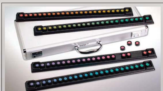
The X-Rite Farnsworth-Munsell 100 Hue Color Vision Testing kit, consists of four trays containing 85 color caps to test the subject.
