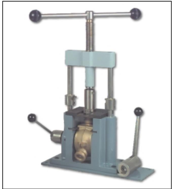
Allow the flask to remain in the press for 60 seconds, then remove it and continue processing in your normal manner for the acrylic used. As you will realize, at this time, if all steps have been followed correctly, then you cannot have an open bite. The acrylic you have just injected is subject to 5 times the pressure of conventional packing without the release of pressure, which occurs each time you trial pack in conventional system.
